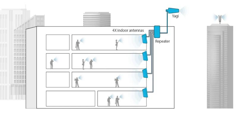
An external antenna installed on the roof of the building receives the signal from all mobile operators.
