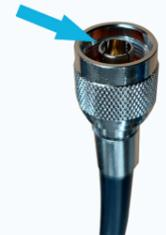
Centre pin must be level with the steel collar. Not pushed inside.
