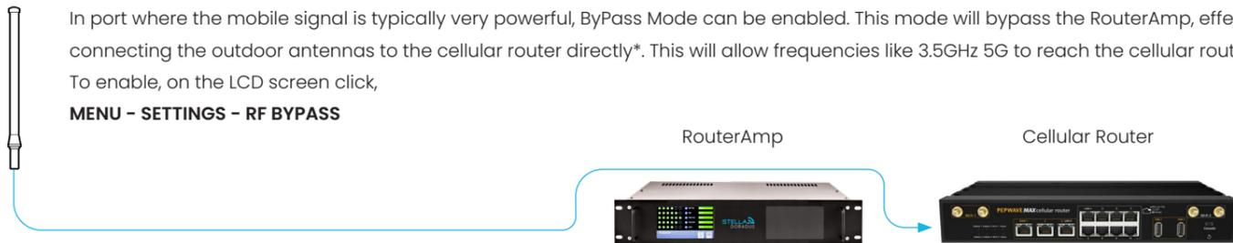
\*ByPass mode introduces 7dB loss to the channel. In practice this loss is easily overcome by the strong signal in port.
